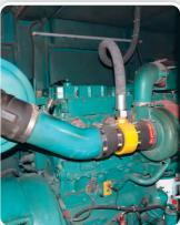
During Dual Fuel operation, a reduced quantity of diesel fuel acts as the ignition source for the air-gas mixture. The Methane rich gas mix replaces significant proportion of Diesel to produce equivalent heat energy during combustion in the cylinder. The emission from such engines see an order of improvement. In the current market conditions this also means significant reduction in cost.
